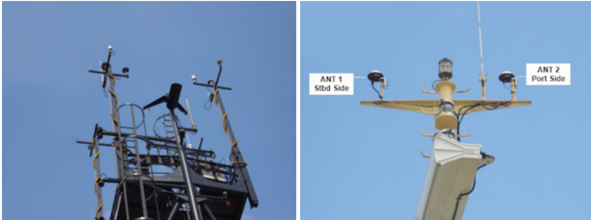
Examples of good installations – Antennas placed at top of mast with good spacing
