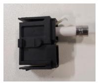
Figure 4 Extracted Fuse Holder
