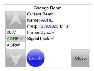
When the required beam name is highlighted, touch the *Enable* button, and then *Close*.
