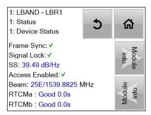
Confirm 'Frame Sync', 'Signal Lock' and beam settings for the selected beam.
