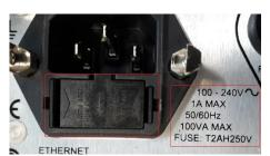
Figure 1 Fuse Holder and Rating
