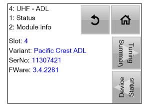
Displays the UHF card serial number and firmware version.
