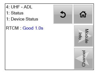
Displays the time in seconds elapsed from the last RTCM string received.
