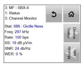
A typical MF channel values range is shown in the screen above.
