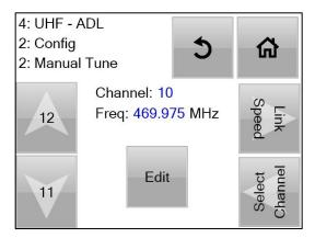
Select using the Arrows to show the required Channel number then press the *Edit* button.
