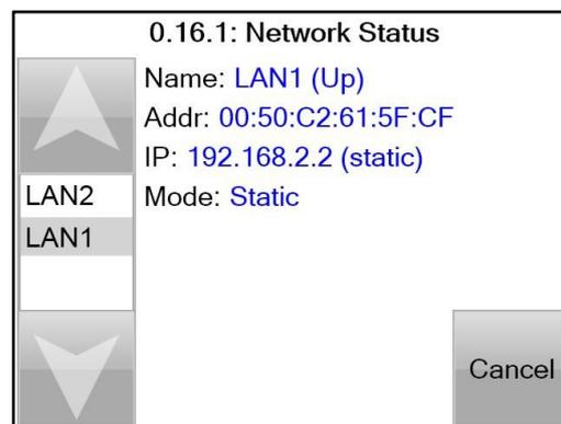
The **Up/Down** arrows may be used to switch between LAN1 and LAN2. The following information is displayed:
