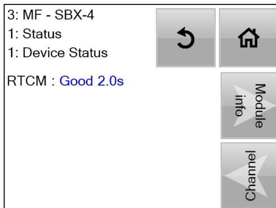
The RTCM entry shows the correction age in seconds. In normal use this will correct every few seconds.
