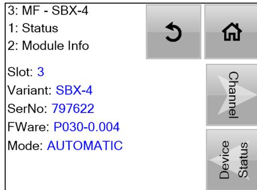
This gives information on whether the MF receiver is in AUTOMATIC or MANUAL mode as well as the serial and firmware numbers for the SBX-4 MF receiver card.
