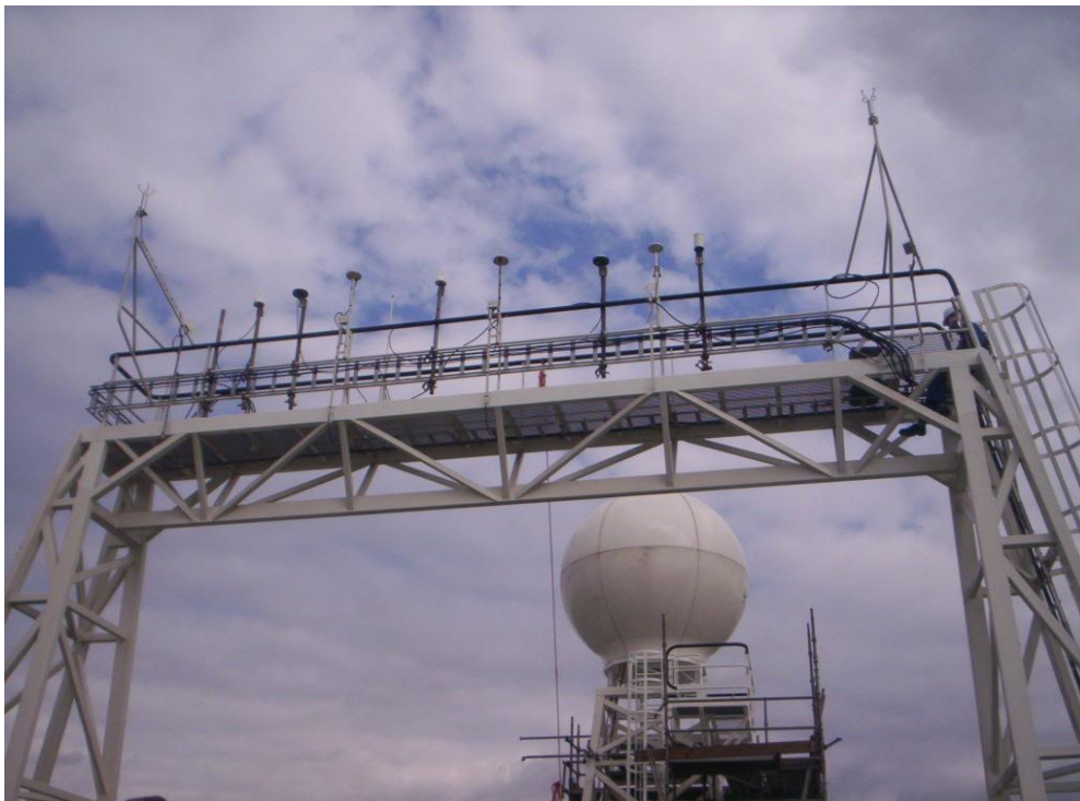
Antennas properly spaced at the same height with only minor signal masking from anemometers.
