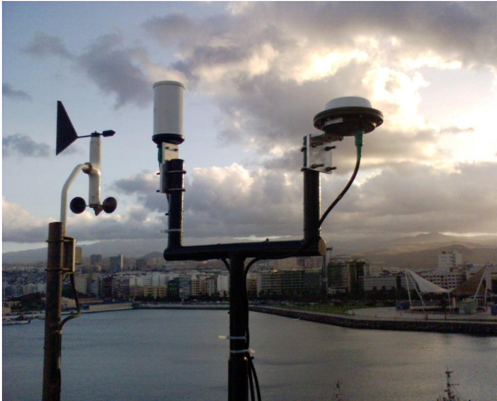
AD410 GNSS antenna and 90984 L-Band Antenna installed on navigation mast with clear 360deg view of sky. Minor GNSS signal masking by the 90984 is present, but only at low satellite elevations.
