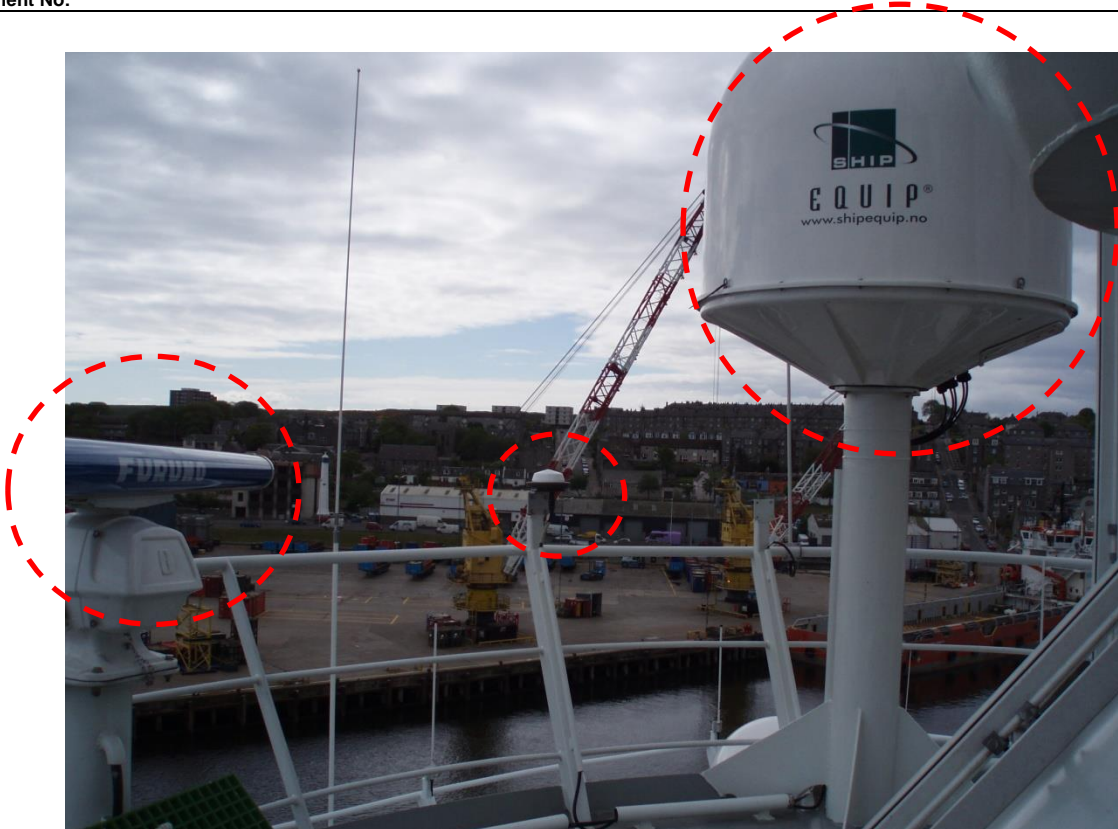
AD410 GNSS antenna installed beneath Sat-B dome and in direct path of RADAR transmissions ; signal masking and interference experienced.
