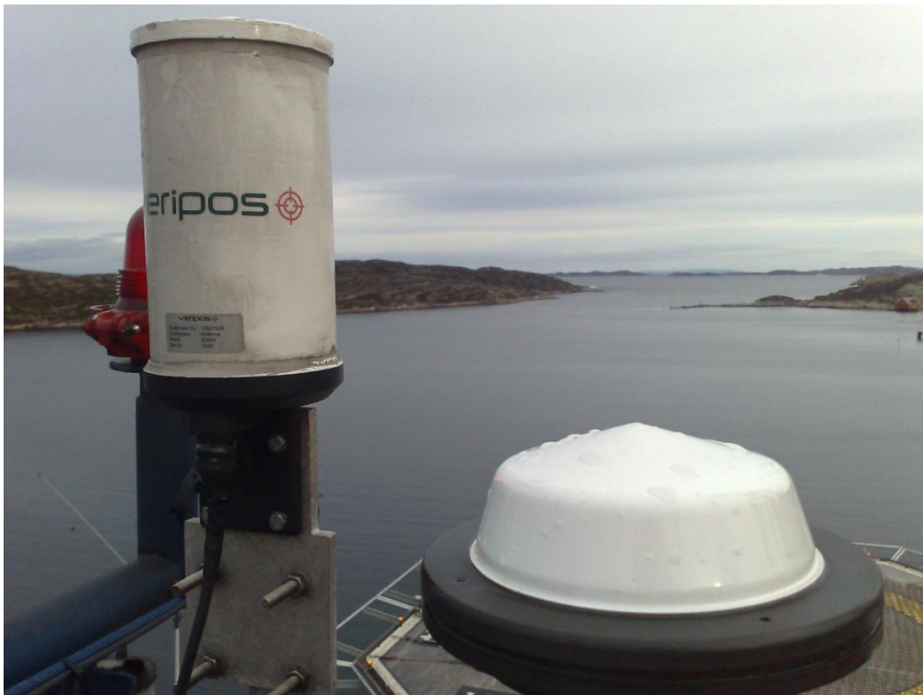
Antennas installed in very close proximity. Ray dome of AD410 GNSS antenna is level with ground plane of 90984 L-Band antenna; signal masking experienced.
