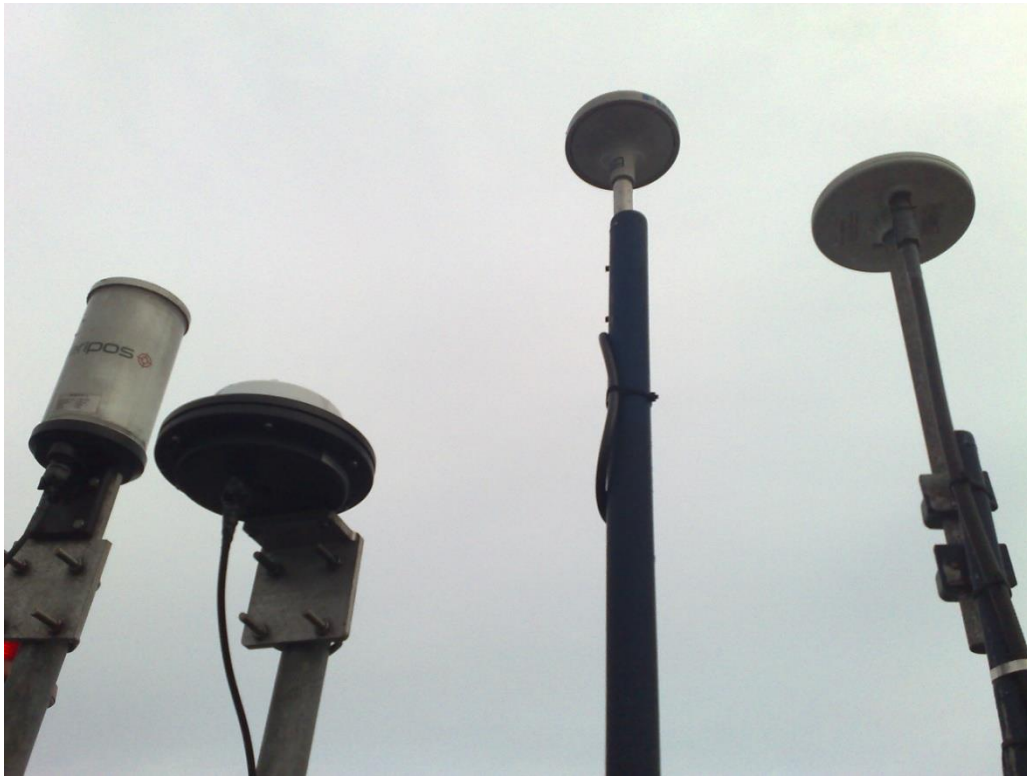
Antennas installed in very close proximity; signal masking experienced.
