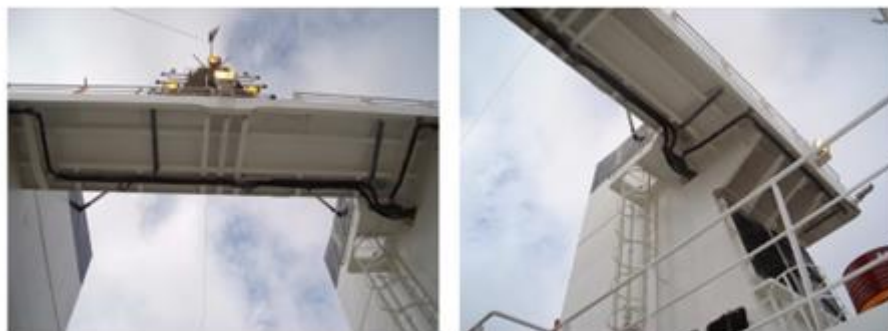
Figure 20. Typical Cable Installation in Bridge and Mast Area
