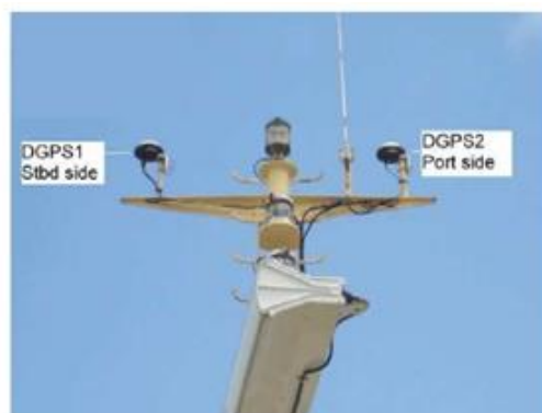
Fig 12. Good Installation – GNSS Antennas Installed on top of the Mast, Minor Signal Masking from Mast Light at low Elevations
