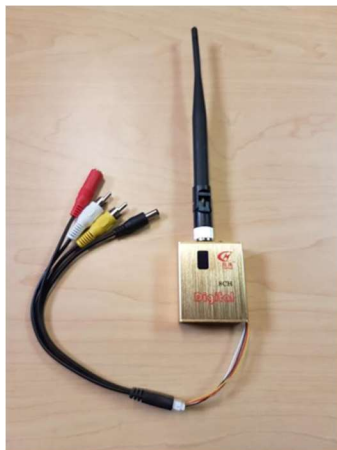
Figure 17: Video transmitter for a drone used as an L2 interference source
