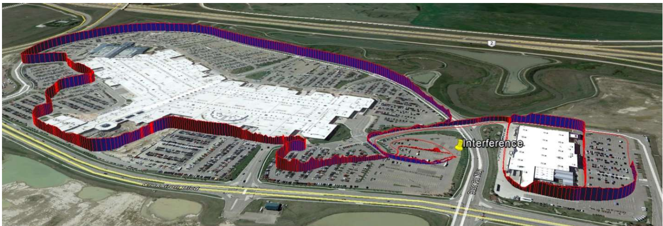
Figure 19: Number of L2 satellites tracked (red) over the test course (Map data: Google, Landsat / Copernicus, DigitalGlobe)
