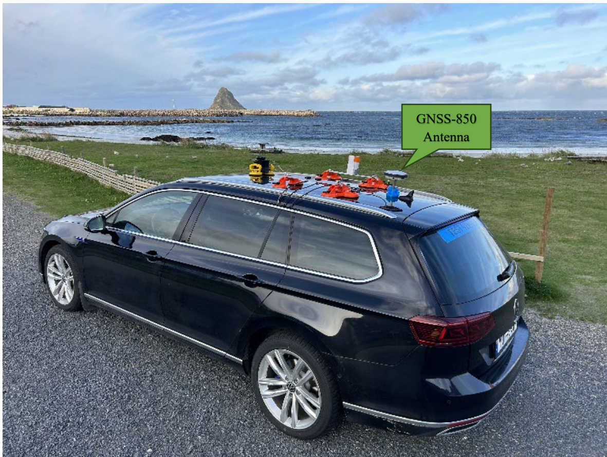
Figure 3 NovAtel's test vehicle with GNSS-850 antenna on the roof
