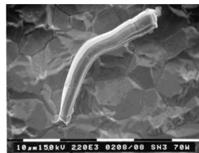
Tin whisker electron micrograph, showing the behaviour of the filament to grow at right angles to the plated surface. Photograph courtesy of EFSOT (Environmentally Friendly Soldering Technologies), www.efsot-europe.info
