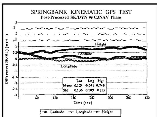
**Figure 5-I-Semikin Dynamic Positions vs C<sup>3</sup>NAV Code/Phase Positions**
