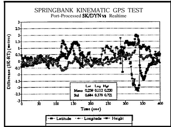
**Figure 5-Semikin Dynamic Positions vs Real-Time Positions**
