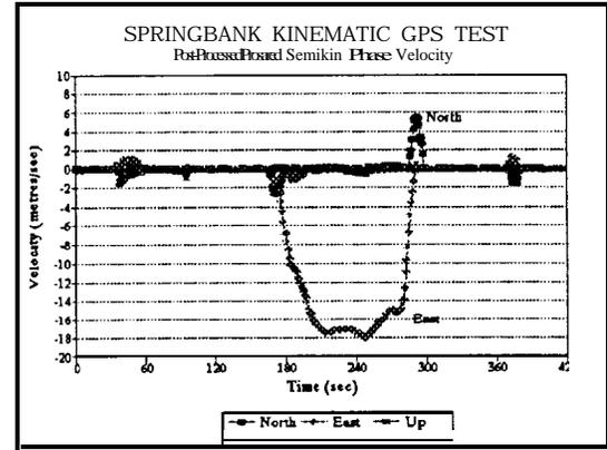
**Figure 6-Semikin Phase Derived Velocity**
