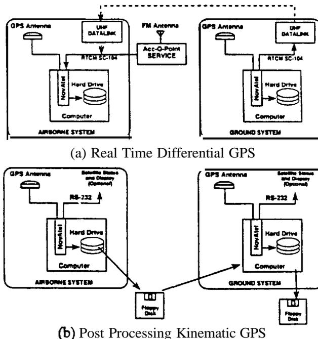
Figure 2. System Configuration
