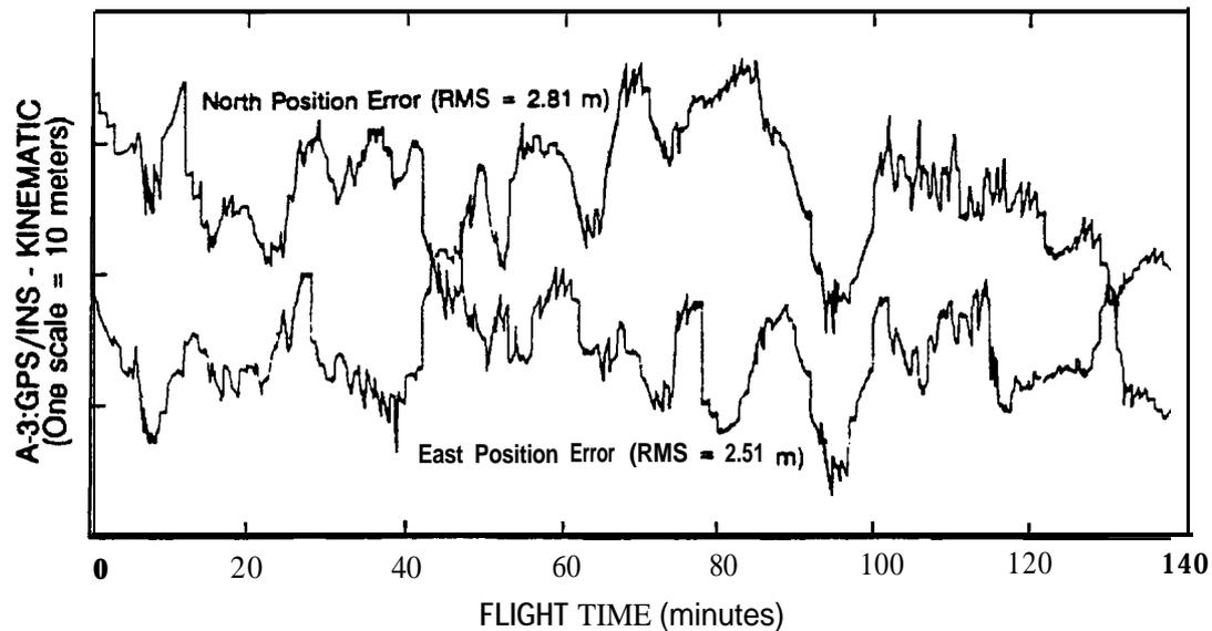
Figure 14. Position Differences between Kinematic and A-3 GPS/INS Navigation Suite
