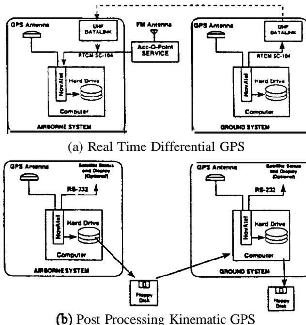
Figure 2. System Configuration
