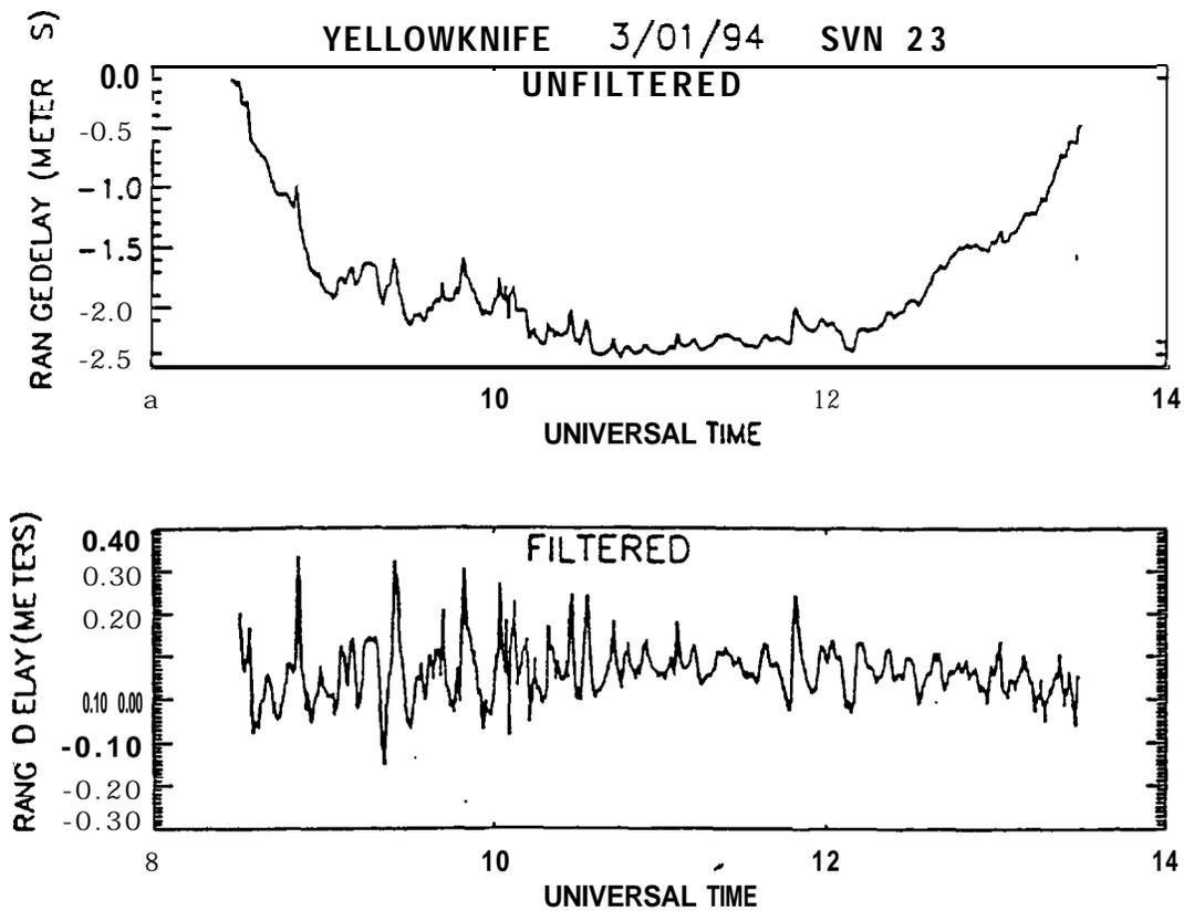
Figure 3. Ionospheric delay variations, before and after removal of low frequency spectral components.
