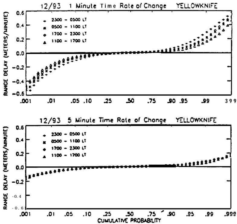
Figure 5. Statistics of ionospheric delay variations over 1 minute and 5 minute periods for different times of day.
