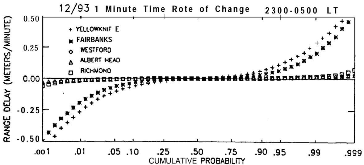
Figure 7. Statistics of ionospheric delay variations for nighttime hours for the stations indicated.
