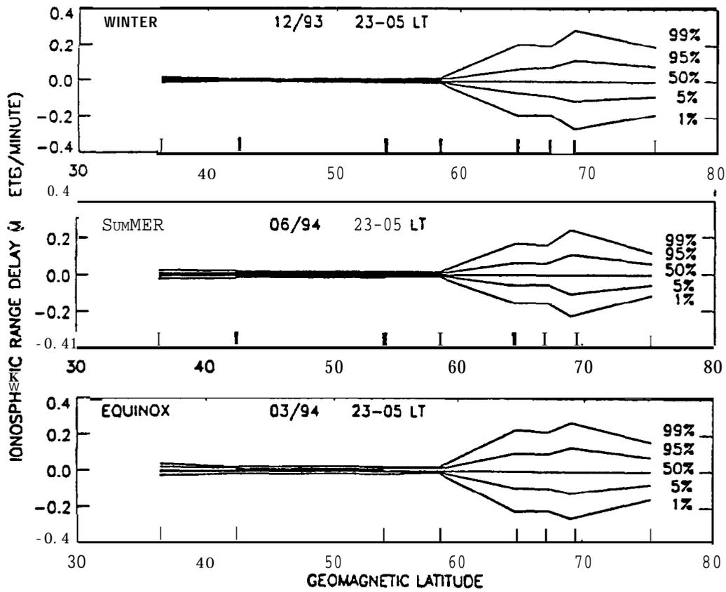
Figure 11. Summary of statistics of nighttime ionospheric delay variations for different seasons versus geomagnetic latitude.
