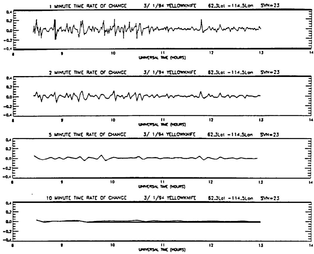
Figure 4. Ionospheric delay variations over the time intervals indicated.
