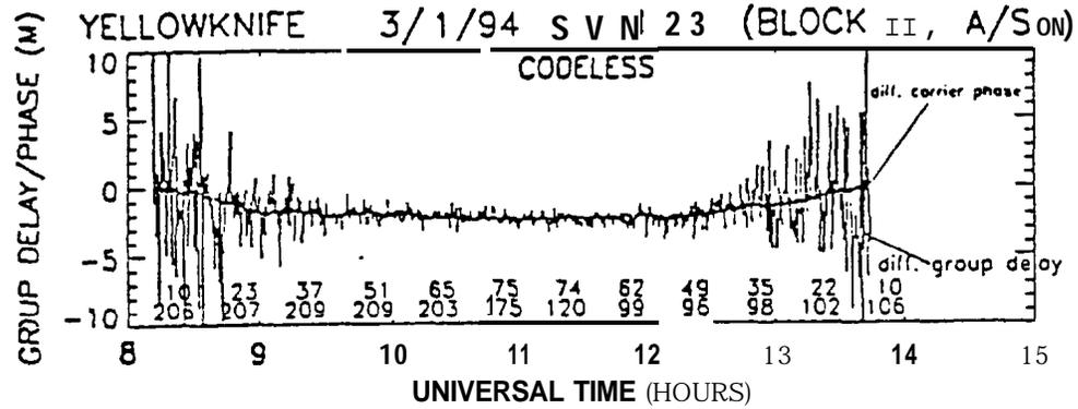
Figure 2. Differential group delay and differential carrier phase under code and codeless conditions.
