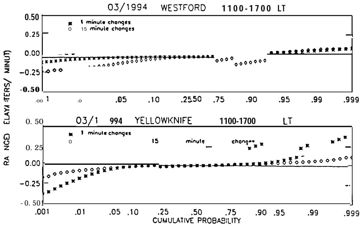
Figure G. Statistics of ionospheric range delay changes for satellite passes from Westford and Yellowknife for which the long period variations were not filtered out.
