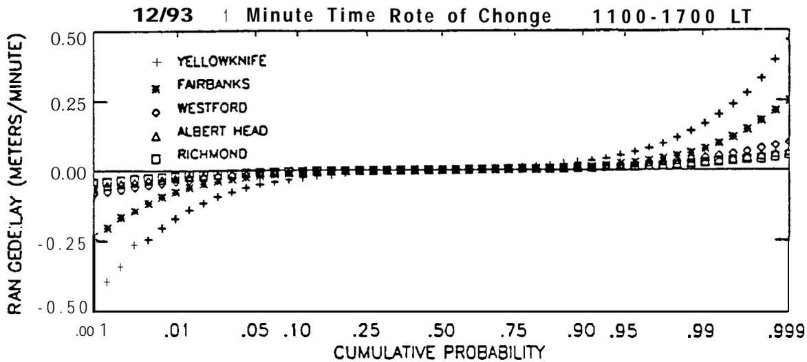
Figure 8. Statistics of ionospheric delay variations for daytime hours for the stations indicated.
