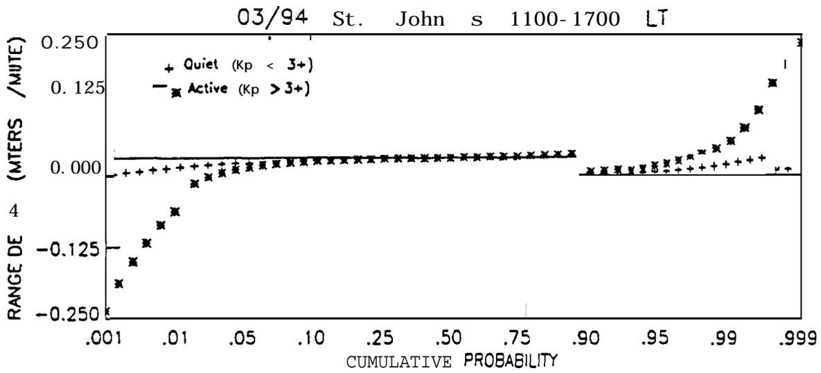
Figure 10. Statistics of daytime ionospheric delay variations for St. Johns, Newfoundland for different conditions of magnetic activity.
