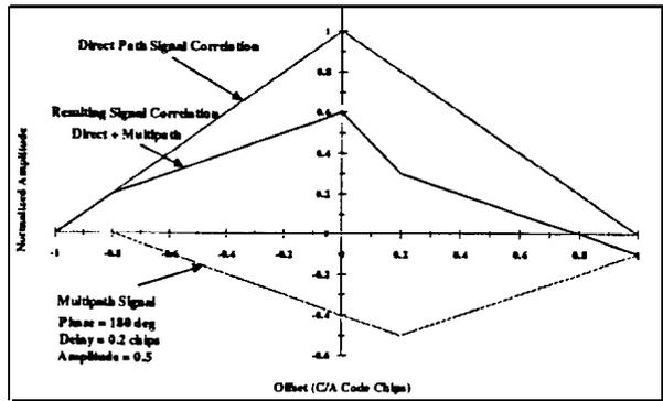
**Figure 6: Direct Path, Multipath ( out of phase) and Resulting Correlation Functions -- Ideal Case**
