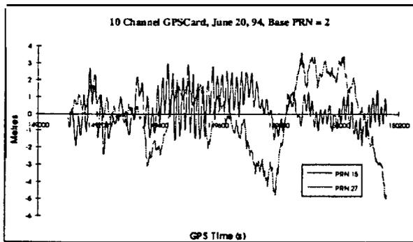
Figure 11: Double Difference Residuals -- Model 951R GPSCards
