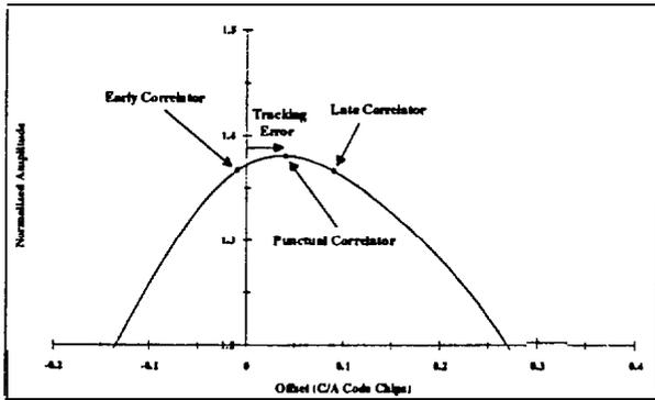
**Figure 4: Tracking Error Due to Multipath**
