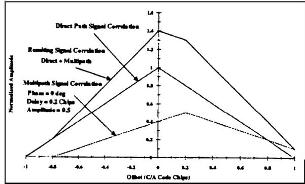
**Figure 5: Direct Path, Multipath ( in phase) and Resulting Correlation Functions -- Ideal Case**
