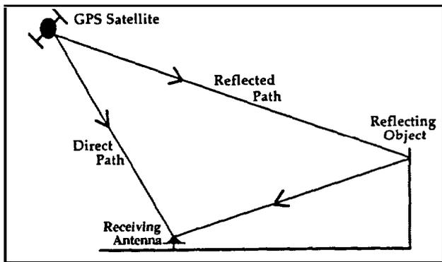
Figure 1: Direct Path and Multipath (Reflected Path) Signals
