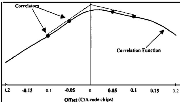
Figure 8: Early Late Slope Technique -- Band Limited Case
