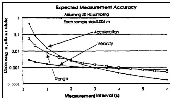
**Figure 2: Expected Accuracy of Filtered Measurements**
