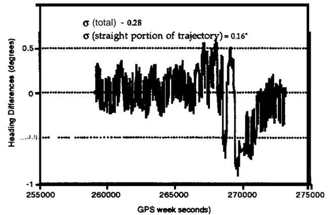
Figure 9: Heading Differences between GPS and Gyrocompass-June 1 Test
