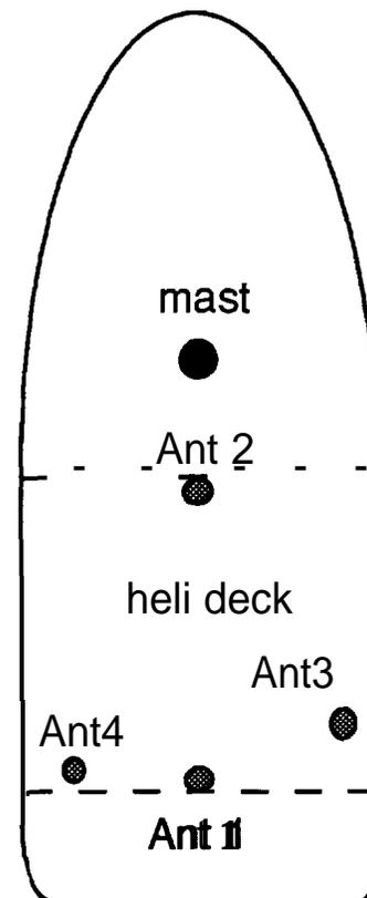
Figure 1: Antenna Layout on Ship
