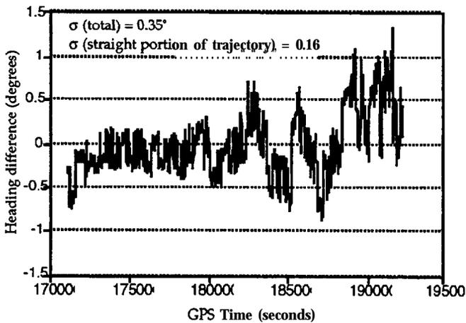
Figure 4: Heading Differences between GPS and Gyrocompass - May 31 Test
