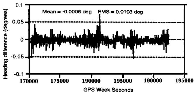
Figure 11: Heading Differences between 4-Antenna and Z-Antenna GPS Attitude System - May 31 Test
