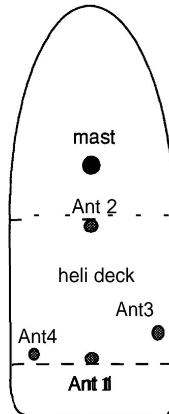
Figure 1: Antenna Layout on Ship
