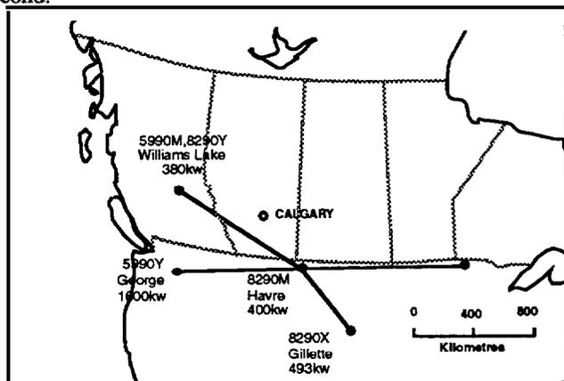
**Figure 1: Loran-C Transmitters Available in Calgary Area**
