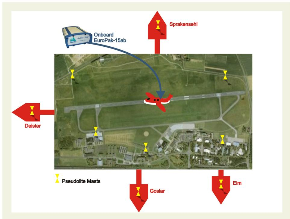
Figure 3: Braunschweig Airstrip and *aviationGATE* Pseudolite Mast Locations
