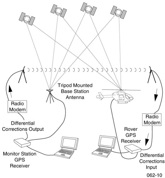
**Figure 1. Basic Components Of ADGPS**
