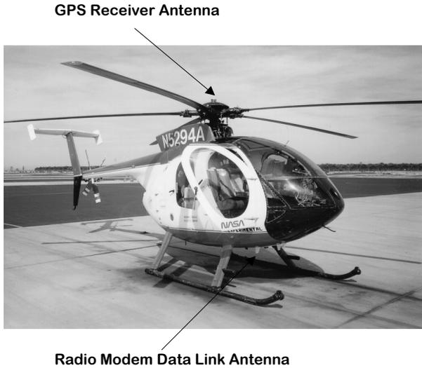
**Figure3. Test Aircraft With Antenna Installations**
