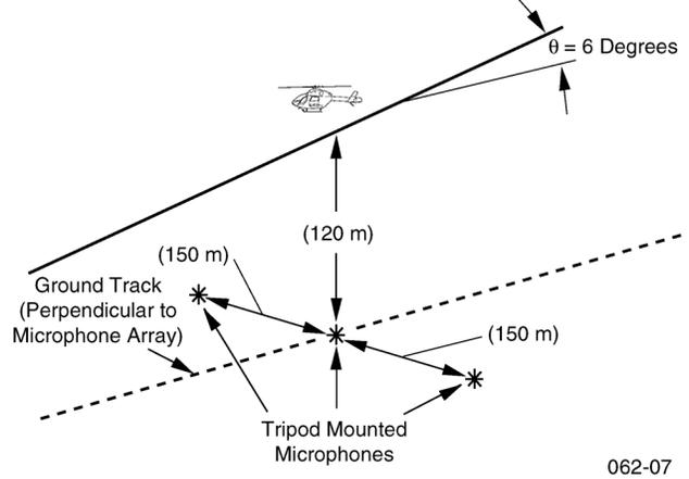
Figure 6. Approach-To-Landing Test Profile
