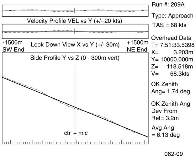
Figure 9. Real-Time Position and Velocity Plot
