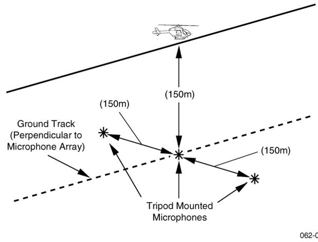
Figure 5. Level Flyover Test Profile
