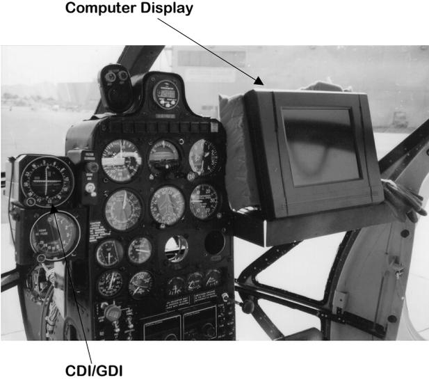
**Figure4. Test Aircraft Instrument Panel**
