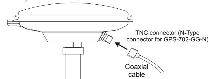
5. Attach the other end of the coaxial cable to the antenna input port of the receiving device, which must provide power as detailed in the *SPECIFICATIONS* section of this guide. All NovAtel GPS receivers provide the necessary power through their antenna RF connectors.
