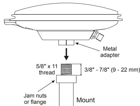
The metal adapter on the bottom of the antenna is fixed in place. Do not attempt to remove it.
