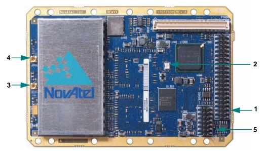
Figure 15: OEMV-3 Connector and Indicator Locations
