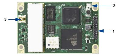
Figure 16: OEMV-1DF Connector and Indicator Locations
