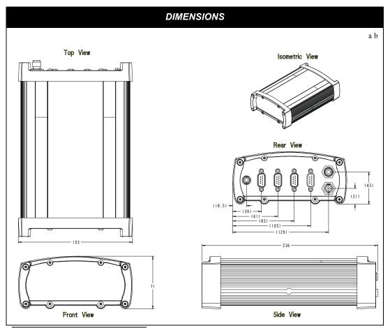
a.All dimension are in millimetres, please use the *Unit Conversion* section of the *GPS+ Reference Manual* for conversion to imperial measurements.
