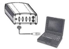
Figure 6: USB Cable Connection
