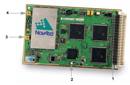
Figure 5: Euro-3 Connector and Indicator Locations
