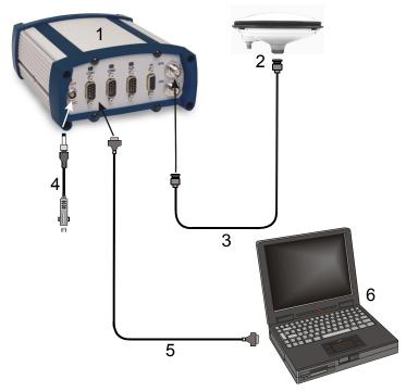
Figure 4: Typical Receiver Installation
