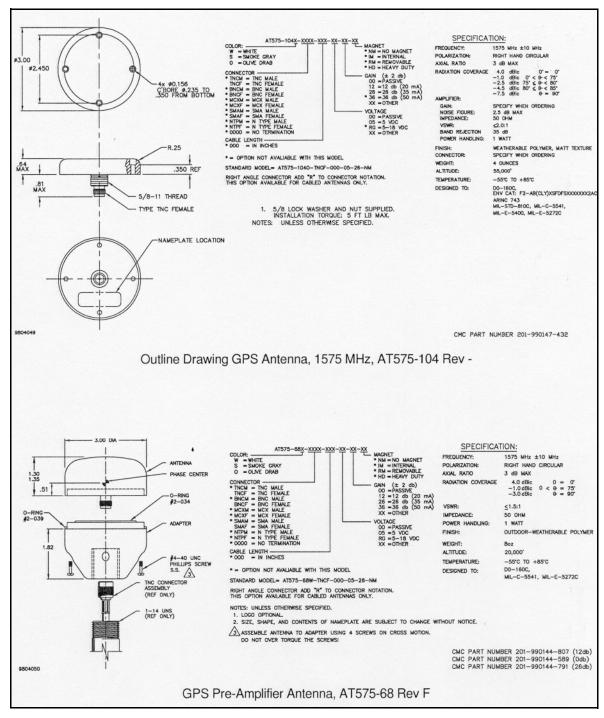
Figure 19: GPS Antenna AT575-104 (1575 MHz) and AT575-68 (Pre-Amplifier)
