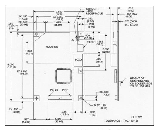
Figure 4: Receiver OEM Board Outline Drawing, VAR XX1
