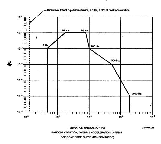
Figure 6: SAE Composite Curve (Random Vibration)
