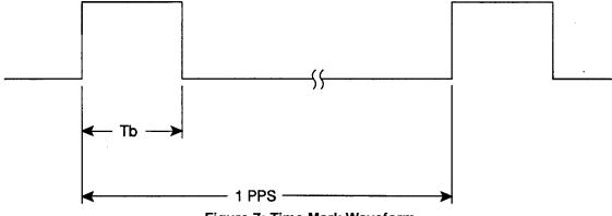
Figure 7: Time Mark Waveform
