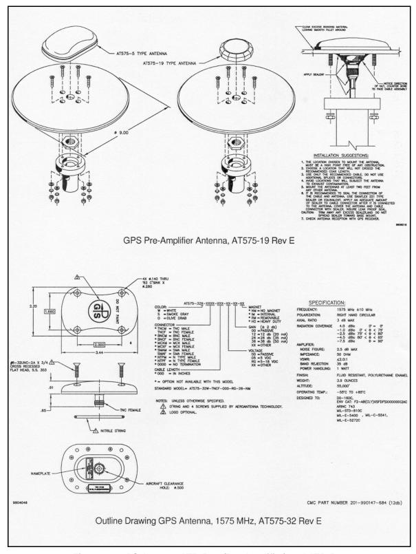
Figure 16: GPS Antenna AT575-19 (Pre-Amplifier) and AT575-32
