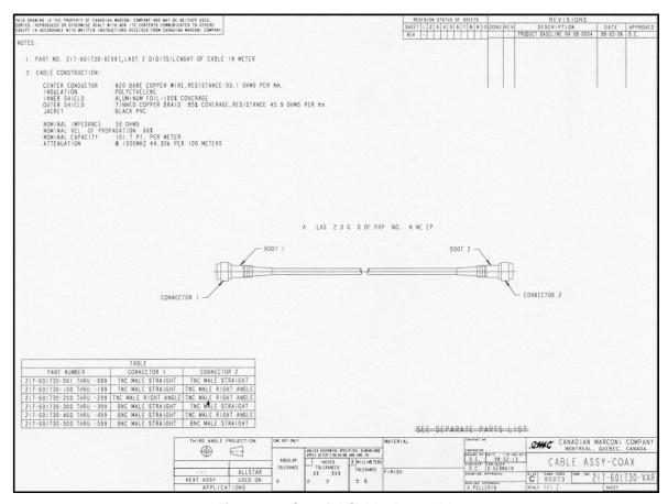
Figure 20: Coaxial Cable Assembly
