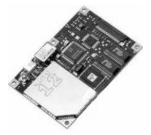
Figure 1: Receiver Single Board
