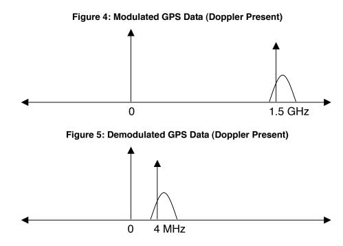
Because of the doppler shift, the reconstructed carrier is shifted in frequency. We reconstitute a frequency of Fnom + Fdoppler
