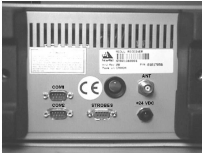
**Figure 4** Rear Panel of Portable MEDLL Receiver
