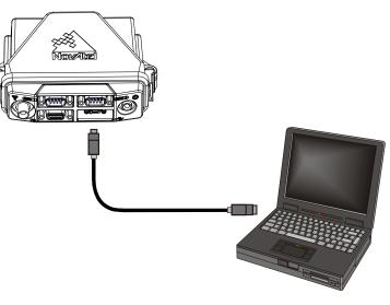
4. Connect the power cable connector to the *PWR* port. Line up the red mark on one power cable connector with the red mark on the receiver's PWR port and insert power cable.
