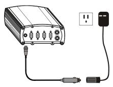
5. Plug in the adapter and/or connect and turn on the power supply. The LED above the PWR port glows red when the EuroPak is properly powered.
