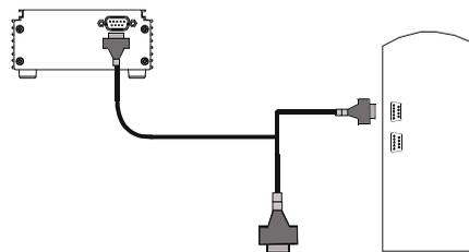
4. Connect the power cable to the power port, which is labeled *10 - 36V DC*.
