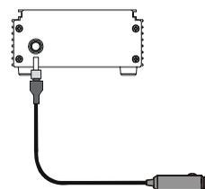
5. Plug in the adapter and/or connect and turn on the power supply. When the PowerPak is properly powered, the *POWER LED* will be red.
