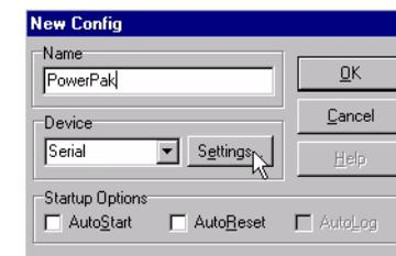
6. Select the PC serial port the PowerPak is connected to from the *PC Port* drop-down list.
