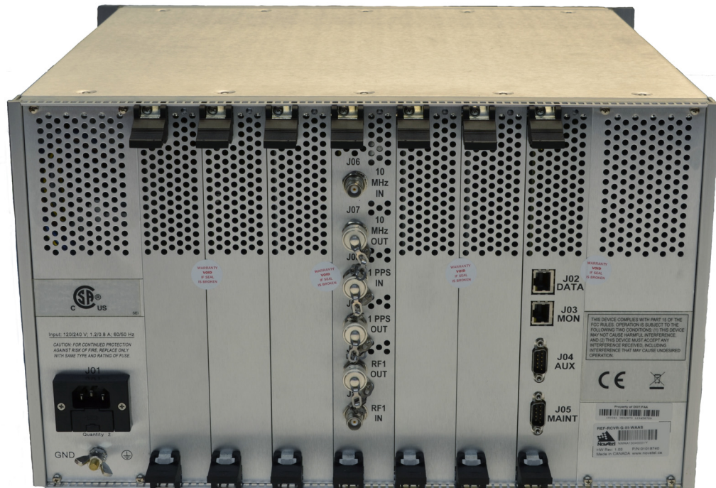
Figure 4: G-III Reference Receiver back panel
