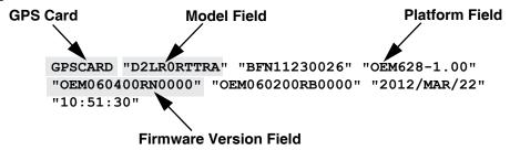
In this example, the last character in the model field ends with an "A" and the firmware version field reads "OEM060400RN0000", therefore an application can be loaded and executed on the receiver. If an update to the firmware and/or model is needed, instructions are provided in Section 3.1.2 and Section 3.1.3 of this document.
