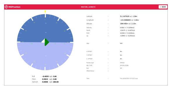
The dial is a graphical display of the Roll, Pitch and Azimuth values indicated by an arrow on each axis. These values appear under the dial.
