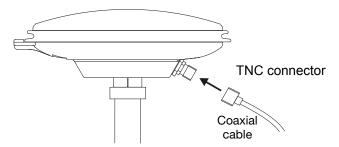
Attach the other end of the coaxial cable to the antenna input port of the receiving device.
