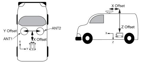
The measurements for the translational offsets should be done as accurately as possible, preferably to within millimeters especially for RTK operation. Any error in the offsets will translate into an error in the INS position.
