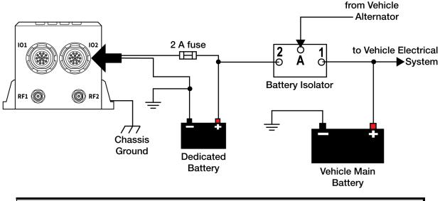
Power can be connected to either the IO1 or IO2 port.
