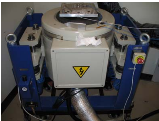
Figure 1 DS2200 Vibration System
