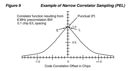
NovAtel's Narrow Correlator tracking technology is "dynamically adjustable". This means that the correlator spacing is initially wide for fast acquisition and reacquisition purposes (1 chip spacing), followed by a narrowing down to 0.1 chip spacing for higher accuracy tracking and multipath rejection.
