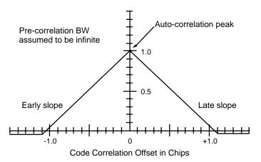
The auto-correlation peak is maintained by continually adjusting the locally generated code for peak correlator output. The unlimited BW provides a sharp correlation peak and steep early/late slope which facilitates accurate error correction for the code-lock-loop (also called Delay Lock Loop).
