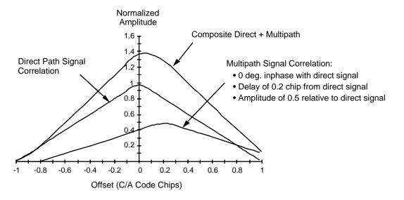
In this example, the multipath signal has a delay of 0.2 chips, an amplitude of 0.5 relative to the direct path signal, and is inphase with the direct path signal. As can be seen by the composite correlation, signal magnitude increases, and more
