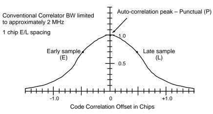
As the E and L correlator samples are spaced 1 chip apart, this places them on the steepest part of the autocorrelation E and L slopes. This placement provides greater sensitivity to changes in the correlation delay-lock-loop (DLL). The E and L samples are differenced to create the appropriate DLL loop feedback for maintaining code lock. Thus, when the E-L difference is zero, the P correlation will be at its peak.
