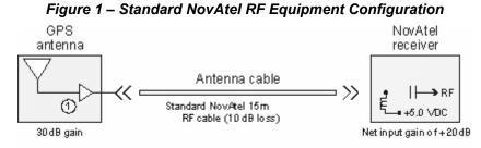
$\bigodot$  The antenna LNA is powered by +5.0 VDC from the receiver via the antenna Cable center conductor.
