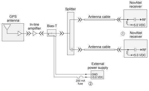
Figure 9 – Single Antenna to Multiple Receivers with In-Line Amplifier
