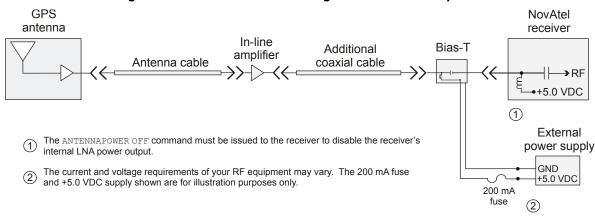
Figure 11 – Additional Cable Length with In-Line Amplifier
