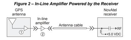
(1) Most GPS antenna LNAs safely operate with +5.0 VDC input voltage.
