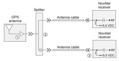
(1) Most GPS antenna LNAs safely operate with +5.0 VDC input voltage.
