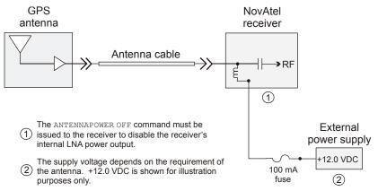
To create this configuration, first connect an external DC power source to the LNA power input pin. The pin number and voltage requirements for the external LNA power input are given in *Table 5* for each receiver type<sup>3</sup>.
