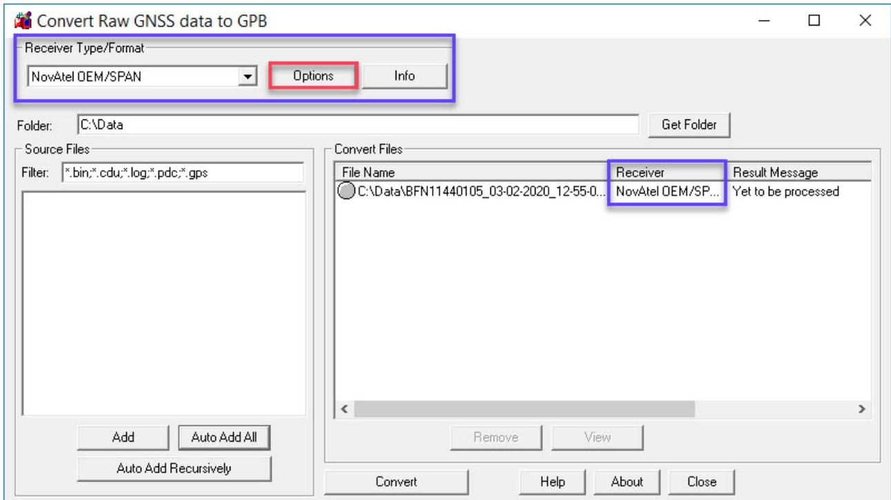
A number of logs, specified in the Recommended Logs list, are used to generate real time trajectory files during data conversion. After the raw data file is added, click the *Options* button, and select the *Create trajectory files for supported records* option. After the data has been converted, the trajectory files can be loaded and viewed in Inertial Explorer, to compare against the post-processed solutions.
